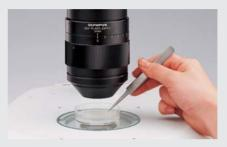
2x objectives with ease of access and correction collar A highly flexible design assures a wide access angle to objectives with the highest NA (0.3) for specimen selection. An additional correction collar can adjust image quality independently of the specimen — a first in stereomicroscopes.
