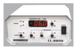
The CL-8800 Temperature Controller can be PREPROGRAMMED with up to 16 temperature programs. It is also PROGRAMMABLE when operated with a computer (IBM compatible) using our proprietary software (CryoGenesisTM V4 and V5 only). It includes a temperature logging module and allows actual temperature progress to be monitored and recorded in the computer (when used).
